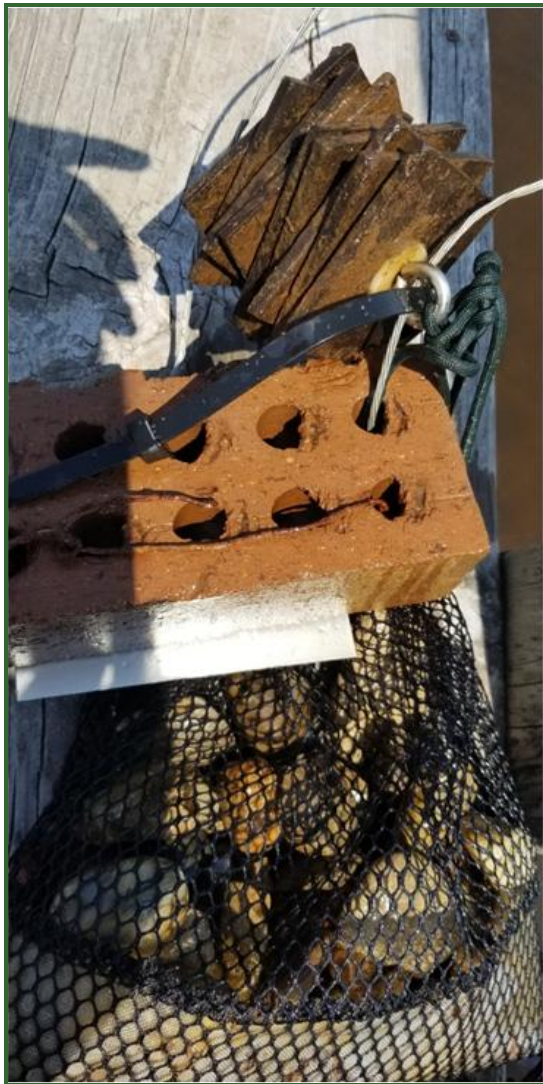
Image (Left): A typical macroinvertebrate sampling array for use in collecting EDRR data pertaining to invasive macroinvertebrates.
