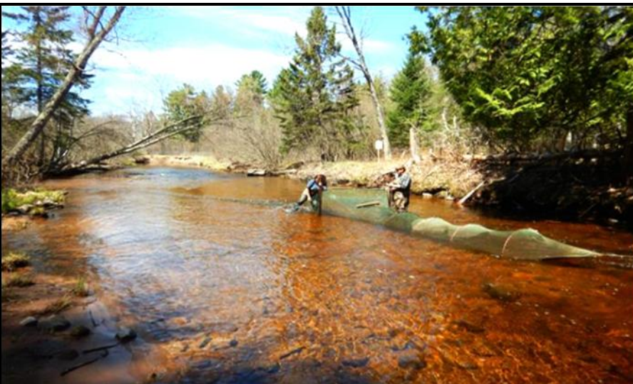
Adult Sea Lamprey Riverine Fyke Net, deployed to capture upstream migrating and spawning phase Sea Lamprey as they ascend rivers, build nests, spawn, and eventually die. The goal is to estimate total numbers of adults in target survey rivers, so total lamprey egg production potential can also be estimated, river to river.
